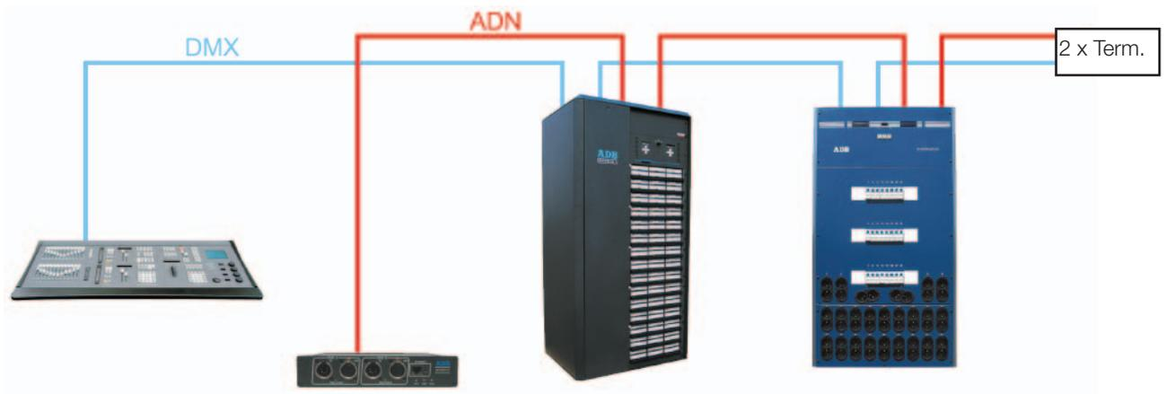
**Example No. 4:** the DMX console is in the control room, at one end of the daisy-chain. NETPORT XT is inserted in the daisy-chain e.g. on stage. In the control room you must terminate the second data pair (pin 4 and 5). And at the other end of the DMX+ADN line you must terminate both data pairs.
