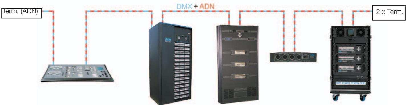
**Note:** the active DMX output of the lighting console (or a DMX amplifier/booster/splitter) replaces the termination for the DMX pair at that end. But you still have to terminate the ADN pair at that end. A very practical tool is a XLR5M-to-XLR5F with internal resistor (120 Ohm) between pins 4 and 5.
