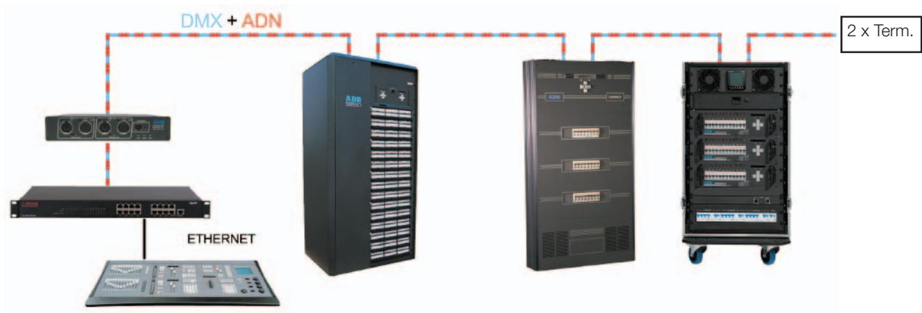
**Example No. 6:** the NETPORT XT is inserted in the daisy-chain e.g. on stage. You must terminate both data pairs at both ends.
