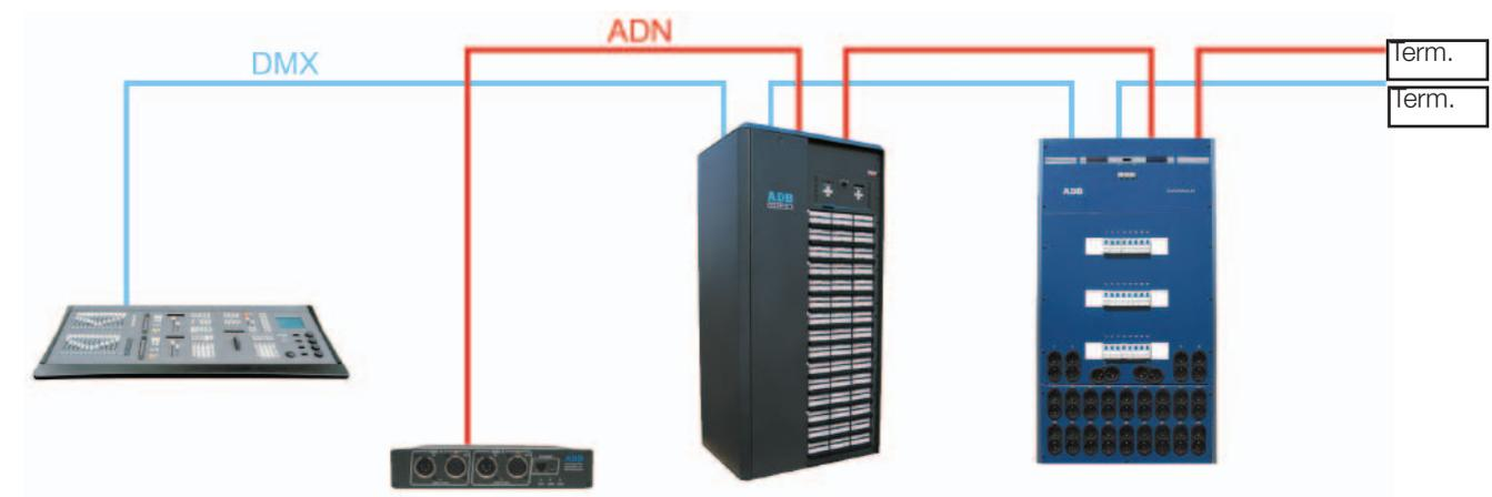
**Example No. 2:** the NETPORT XT is inserted in the daisy-chain e.g. on stage. You must terminate the ADN data pair at both ends.
